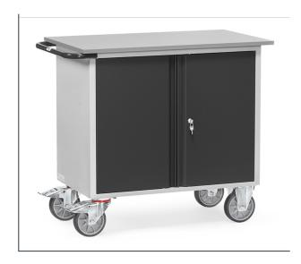
Sectional steel construction. Worktop composite panel grey 20 mm. With 1 cupboard with double door without separation wall. 2 adjustable shelves. Maximum opening angle 120°. Capacity per shelve 80 kg. 2 swivel and 2 fixed-wheel castors, TPE tyres, hubs with groove ball bearing. Swivel castors with wheel locks, according to the European Standard EN 1757-3 (safety of platform trolleys).
