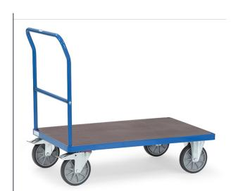
Tubular steel and profile steel welded, powder coated, surface durably protected, resistant to impact and scratches. Platform with nonslip plywood board. 2 swivel and 2 fixed-wheel castors, TPE tyres, hubs with groove ball bearing. Swivel castors with wheel locks, according to the European Standard EN 1757-3 (safety of platform trolleys).
