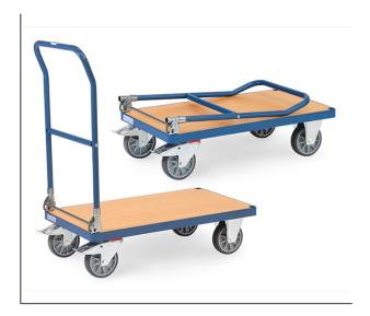
Tubular steel and profile steel welded, powder coated, with platform made of derived timber material boards. Surface beech grain. Handlebar foldable onto platform. 2 swivel and 2 fixed-wheel castors, TPE tyres, hubs with groove ball bearing. Swivel castors with wheel locks, according to the European Standard EN 1757-3 (safety of platform trolleys).
