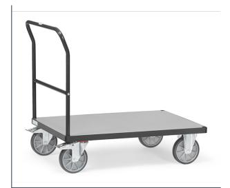
Tubular steel and profile steel welded, powder coated, surface durably protected, resistant to impact and scratches. Platform made of derived timber material boards, surface grey. 2 swivel and 2 fixed-wheel castors, TPE tyres, hubs with groove ball bearing. Swivel castors with wheel locks, according to the European Standard EN 1757-3 (safety of platform trolleys).
