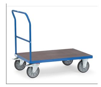
Tubular steel and profile steel welded, powder coated, surface durably protected, resistant to impact and scratches. Platform with nonslip plywood board. 2 swivel and 2 fixed-wheel castors, TPE tyres, hubs with groove ball bearing. Swivel castors with wheel locks, according to the European Standard EN 1757-3 (safety of platform trolleys).
