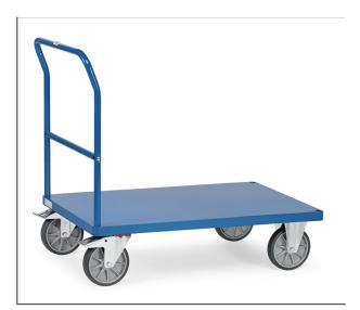
Tubular steel and profile steel welded, powder coated, surface durably protected, resistant to impact and scratches. Platform made of sheeet steel, flush with frame, welded powder coated RAL 5007. 2 swivel and 2 fixed-wheel castors, TPE tyres, hubs with groove ball bearing. Swivel castors with wheel locks, according to the European Standard EN 1757-3 (safety of platform trolleys).
