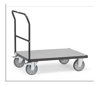
Tubular steel and profile steel welded, powder coated, surface durably protected, resistant to impact and scratches. Platform made of derived timber material boards, surface grey. 2 swivel and 2 fixed-wheel castors, TPE tyres, hubs with groove ball bearing. Swivel castors with wheel locks, according to the European Standard EN 1757-3 (safety of platform trolleys).
