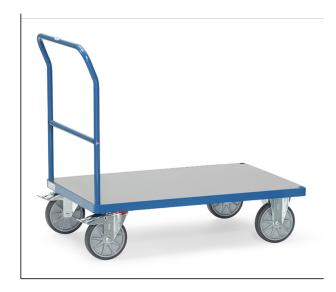
Tubular steel and profile steel welded, powder coated, surface durably protected, resistant to impact and scratches. Platform with weatherproof rigid PVC panel in dark grey. High chemical resistance, low flammability. 2 swivel and 2 fixed-wheel castors, TPE tyres, hubs with groove ball bearing. Swivel castors with wheel locks, according to the European Standard EN 1757-3 (safety of platform trolleys).
