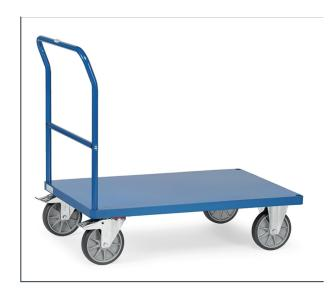
Tubular steel and profile steel welded, powder coated, surface durably protected, resistant to impact and scratches. Platform made of sheeet steel, flush with frame, welded powder coated RAL 5007. 2 swivel and 2 fixed-wheel castors, TPE tyres, hubs with groove ball bearing. Swivel castors with wheel locks, according to the European Standard EN 1757-3 (safety of platform trolleys).
