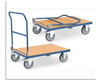
Tubular steel and profile steel welded, powder coated, with platform made of derived timber material boards. Surface beech grain. Handlebar foldable onto platform. 2 swivel and 2 fixed-wheel castors, TPE tyres, hubs with groove ball bearing. Swivel castors with wheel locks, according to the European Standard EN 1757-3 (safety of platform trolleys).
