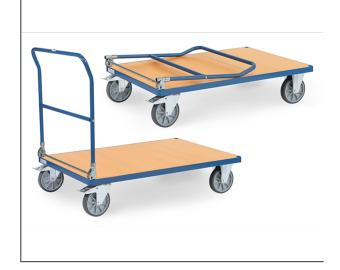
Tubular steel and profile steel welded, powder coated, with platform made of derived timber material boards. Surface beech grain. Handlebar foldable onto platform. 2 swivel and 2 fixed-wheel castors, TPE tyres, hubs with groove ball bearing. Swivel castors with wheel locks, according to the European Standard EN 1757-3 (safety of platform trolleys).
