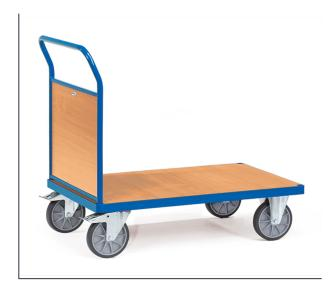
Tubular steel and profile steel welded, powder coated, surface durably protected, resistant to impact and scratches. Platform and panelled end made of derived timber material boards, surface beech grain. Height of panelled end 500 mm. 2 swivel and 2 fixed-wheel castors, TPE tyres, hubs with groove ball bearing. Swivel castors with wheel locks, according to the European Standard EN 1757-3 (safety of platform trolleys).
