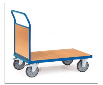
Tubular steel and profile steel welded, powder coated, surface durably protected, resistant to impact and scratches. Platform and panelled end made of derived timber material boards, surface beech grain. Height of panelled end 500 mm. 2 swivel and 2 fixed-wheel castors, TPE tyres, hubs with groove ball bearing. Swivel castors with wheel locks, according to the European Standard EN 1757-3 (safety of platform trolleys).
