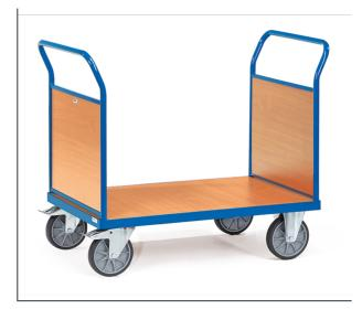
Tubular steel and profile steel welded, powder coated, surface durably protected, resistant to impact and scratches. Platform and panelled ends made of derived timber material boards, surface beech grain. Height of panelled ends 500 mm. 2 swivel and 2 fixed-wheel castors, TPE tyres, hubs with groove ball bearing. Swivel castors with wheel locks, according to the European Standard EN 1757-3 (safety of platform trolleys).
