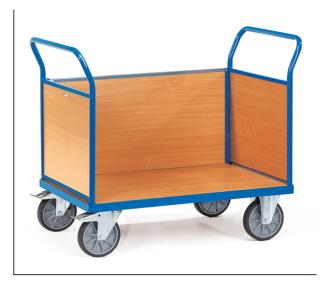
Tubular steel and profile steel welded, powder coated, surface durably protected, resistant to impact and scratches. Platform, panelled ends and 1 panelled side made of derived timber material boards, surface beech grain. Height of panelled ends and side 500 mm. 2 swivel and 2 fixed-wheel castors, TPE tyres, hubs with groove ball bearing. Swivel castors with wheel locks, according to the European Standard EN 1757-3 (safety of platform trolleys).
