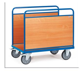
Tubular steel and profile steel welded, powder coated, surface durably protected, resistant to impact and scratches. Platform made of derived timber material boards, surface beech grain. Sides made of derived timber material boards, surface beech grain. Height of sides 600/750 mm. 2 swivel and 2 fixed-wheel castors, TPE tyres, hubs with groove ball bearing. Swivel castors with wheel locks, according to the European Standard EN 1757-3 (safety of platform trolleys).
