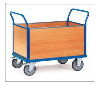
Tubular steel and profile steel welded, powder coated, surface durably protected, resistant to impact and scratches. Platform, panelled ends and panelled sides made of derived timber material boards, surface beech grain. With one detachable side. Height of panelled ends and sides 500 mm. 2 swivel and 2 fixed-wheel castors, TPE tyres, hubs with groove ball bearing. Swivel castors with wheel locks, according to the European Standard EN 1757-3 (safety of platform trolleys).
