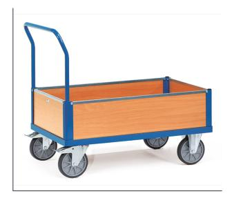
Tubular steel and profile steel welded, powder coated, surface durably protected, resistant to impact and scratches. Platform made of derived timber material boards, surface beech grain. Ends and sides made of derived timber material boards. Height of sides 250 mm. All sides singly detachable. 2 swivel and 2 fixed-wheel castors, TPE tyres, hubs with groove ball bearing. Swivel castors with wheel locks, according to the European Standard EN 1757-3 (safety of platform trolleys).
