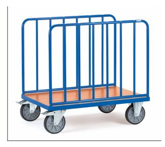
Tubular steel and profile steel welded, powder coated, surface durably protected, resistant to impact and scratches. Platform made of derived timber material boards, surface beech grain. 2 tubular steel side frames with intermediate uprights at intervals of approx. 130 mm. 2 swivel and 2 fixed-wheel castors, TPE tyres, hubs with groove ball bearing. Swivel castors with wheel locks, according to the European Standard EN 1757-3 (safety of platform trolleys).
