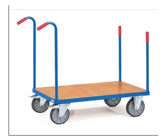
Tubular steel and profile steel welded, powder coated, surface durably protected, resistant to impact and scratches. Platform made of derived timber material boards, surface beech grain. 2 swivel and 2 fixed-wheel castors, TPE tyres, hubs with groove ball bearing. Swivel castors with wheel locks, according to the European Standard EN 1757-3 (safety of platform trolleys).
