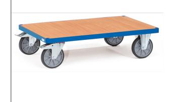
Profile steel welded, powder coated, surface durably protected, resistant to impact and scratches. Platform made of derived timber material boards, surface beech grain. 2 swivel and 2 fixed-wheel castors, TPE tyres, hubs with groove ball bearing. Swivel castors with wheel locks, according to the European Standard EN 1757-3 (safety of platform trolleys).
