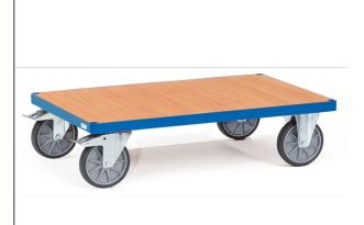
Profile steel welded, powder coated, surface durably protected, resistant to impact and scratches. Platform made of derived timber material boards, surface beech grain. 2 swivel and 2 fixed-wheel castors, TPE tyres, hubs with groove ball bearing. Swivel castors with wheel locks, according to the European Standard EN 1757-3 (safety of platform trolleys).
