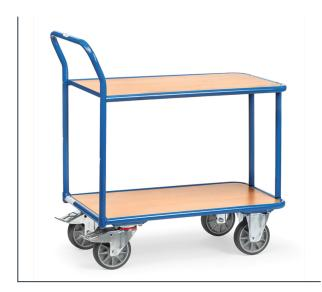
Modular system, platform and pushbar and upper shelf with screw connection. Capacity upper and middle shelf 120 kg. Disassembled on delivery. Welded tubular or sectional steel construction, powder coated, blue RAL 5007. Shelves made of derived timber material board, beech decor surface. 2 swivel and 2 fixed-wheel castors, TPE tyres, hubs with groove ball bearing. Swivel castors with wheel locks, according to the European Standard EN 1757-3 (safety of platform trolleys).
