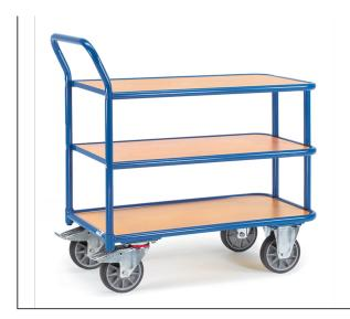
Modular system, platform and pushbar and upper and middle shelf with screw connection. Capacity upper and middle shelf 120 kg. Disassembled on delivery. Welded tubular or sectional steel construction, powder coated, blue RAL 5007. Shelves made of derived timber material board, beech decor surface. 2 swivel and 2 fixed-wheel castors, TPE tyres, hubs with groove ball bearing. Swivel castors with wheel locks, according to the European Standard EN 1757-3 (safety of platform trolleys).
