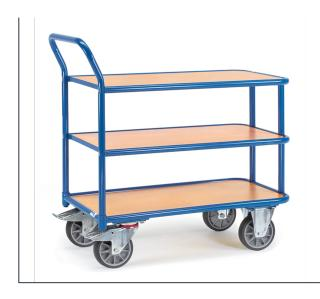
Modular system, platform and pushbar and upper and middle shelf with screw connection. Capacity upper and middle shelf 120 kg. Disassembled on delivery. Welded tubular or sectional steel construction, powder coated, blue RAL 5007. Shelves made of derived timber material board, beech decor surface. 2 swivel and 2 fixed-wheel castors, TPE tyres, hubs with groove ball bearing. Swivel castors with wheel locks, according to the European Standard EN 1757-3 (safety of platform trolleys).
