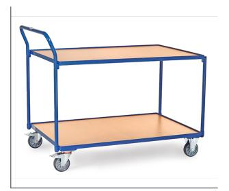
Modular system: Tubular steel welded and powder coated, surface durably protected, resistant to impact and scratches. 2 shelves made of derived timber material boards, in a frame of angle steel, height of rim 12 mm. 2 swivel and 2 fixed-wheel castors, TPE tyres, hubs with groove ball bearing. Swivel castors with wheel locks, according to the European Standard EN 1757-3 (safety of platform trolleys). Capacity upper shelf 80 kg.
