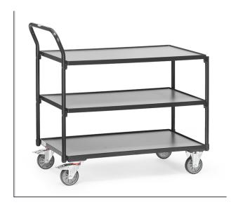
Modular system: Tubular steel welded and powder coated, surface durably protected, resistant to impact and scratches. 3 shelves made of derived timber material boards, in a frame of angle steel, height of rim 12 mm. 2 swivel and 2 fixed-wheel castors, TPE tyres, hubs with groove ball bearing. Swivel castors with wheel locks, according to the European Standard EN 1757-3 (safety of platform trolleys). Capacity upper and middle shelf 80 kg.
