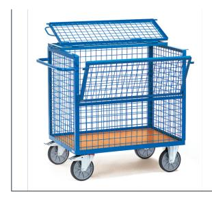
Tubular steel and profile steel welded, powder coated blue RAL 5007. Platform made of derived timber material board, surface beech grain. Wire cage cart with angular steel superstructure, wire lattice 50 x 50 x 4mm, welded. Cover double collapsible. Ring-eyelets for padlocks. Useful height: 806 mm. 2 swivel and 2 fixed-wheel castors, TPE tyres, hubs with groove ball bearing. Swivel castors with wheel locks, according to the European Standard EN 1757-3 (safety of platform trolleys).
