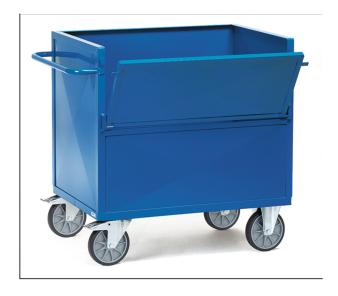
Tubular steel and profile steel welded, powder coated blue RAL 5007. Platforms made of sheet steel, powder coated or galvanized. Sheet steel box cart, angle steel construction, sides made of sheet steel, welded and powder coated. Useful height: 816 mm. 2 swivel and 2 fixed-wheel castors, TPE tyres, hubs with groove ball bearing. Swivel castors with wheel locks, according to the European Standard EN 1757-3 (safety of platform trolleys).
