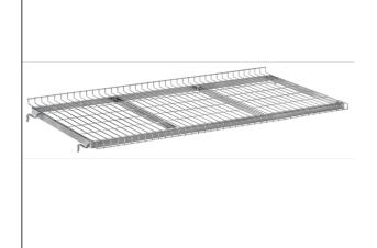
Shelve made of wire lattice with mesh width  $120 \times 30$  mm, electrolytically galvanised. On the long sides with 23 mm upward folded rim, on the other side 23 mm downward folded rim. Variable use of shelves, in a grid of 100 mm horizontal or tilted insertable. Capacity of shelf 40 kg.
