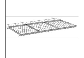
Shelve made of wire lattice with mesh width  $120 \times 30$  mm, electrolytically galvanised. On the long sides with 23 mm upward folded rim, on the other side 23 mm downward folded rim. Variable use of shelves, in a grid of 100 mm horizontal or tilted insertable. Capacity of shelf 80 kg.
