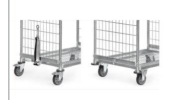
For moving with max. 3 storeroom trolleys in a train. 2 swivel castors without wheel locks will bereplaced by 2 fixed-wheel castors. Shaft made of sheet steel. Shaft raises automatically via gas spring into vertical resting position. Robust coupling pin on the fixed-wheel side. Connection via foot operation possible. Max. train speed 6 km/h. Not combinable with steps.
