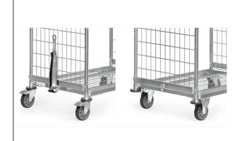
For moving with max. 3 storeroom trolleys in a train. 2 swivel castors without wheel locks will bereplaced by 2 fixed-wheel castors. Shaft made of sheet steel. Shaft raises automatically via gas spring into vertical resting position. Robust coupling pin on the fixed-wheel side. Connection via foot operation possible. Max. train speed 6 km/h. Not combinable with steps.
