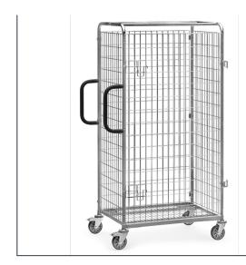
Wing door, wire frame galvanic bright galvanized, mesh width  $100 \times 50$  mm. Hinges can be folded by  $180^{\circ}$  to the car body. 2 wire iron closures lockable by means of padlock (not included).
