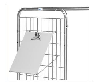
Can be clipped to the wire lattice of side panels, inclination adjustable via support brackets. With paper clamp. Steel sheet, powder coated grey RAL 7035. Effect. size: H x W 335 x 352 mm
