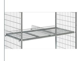
As divider for shelves. With welded clamping lug. Wire lattice, electrolytically galvanised. Size: W x H 506/606 x 95 mm, esh width: 25 mm
