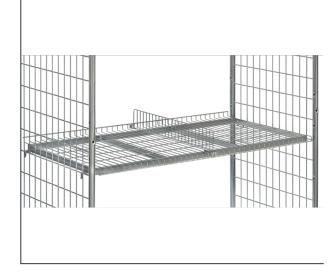
As divider for shelves. With welded clamping lug. Wire lattice, electrolytically galvanised. Size: W x H  $506/606 \times 95$  mm, esh width: 25 mm
