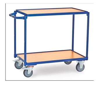
Modular system: Tubular steel welded and powder coated, surface durably protected, resistant to impact and scratches. 2 shelves made of derived timber material boards, in a frame of angle steel, height of rim 12 mm. 2 swivel and 2 fixed-wheel castors, TPE tyres, hubs with groove ball bearing. Swivel castors with wheel locks, according to the European Standard EN 1757-3 (safety of platform trolleys). Capacity upper shelf 80 kg.
