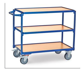
Modular system: Tubular steel welded and powder coated, surface durably protected, resistant to impact and scratches. 3 shelves made of derived timber material boards, in a frame of angle steel, height of rim 12 mm. 2 swivel and 2 fixed-wheel castors, TPE tyres, hubs with groove ball bearing. Swivel castors with wheel locks, according to the European Standard EN 1757-3 (safety of platform trolleys). Capacity upper and middle shelf 80 kg.
