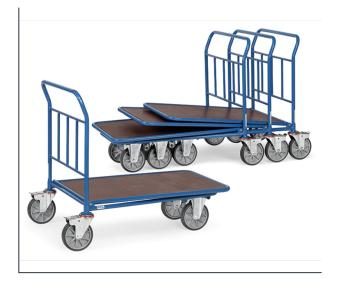
Tubular steel construction, powder coated, platform made of anti-skid waterproof plywood boards. 2 swivel and 2 fixed-wheel castors, TPE tyres. Swivel castors with wheel locks, according to the European Standard EN 1757-3 (safety of platform trolleys).
