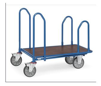
Tubular steel construction, powder coated, platform made of anti-skid waterproof plywood boards. With 2 lateral frames, 680 mm high, on the side of the fixed wheels also 2 lateral frames, 500 mm high. 2 swivel and 2 fixed-wheel castors, TPE tyres. Swivel castors with wheel locks, according to the European Standard EN 1757-3 (safety of platform trolleys).
