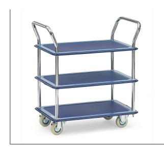
Shelves made of pressed steel plate, powder coated blue RAL 5007, with adhered anti-slip covering and all round protective strip. Tubular push handle. 2 swivel and 2 fixed-wheel castors, solid rubber tyres, hubs with plain bearing. Swivel castors with wheel locks, according to the European Standard EN 1757-3 (safety of platform trolleys). Flat packed delivery.
