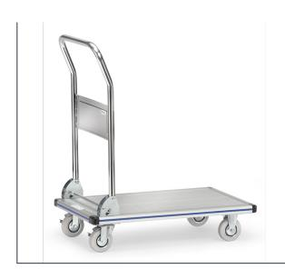
With foldable tubular push handles, closed platform with anti-slip surface, sturdy rounded edge profiles. Tubular push handle with wide strut and sturdy hinged mounting. 2 swivel and 2 fixed-wheel castors, solid rubber tyres, hubs with plain bearing. Swivel castors with wheel locks, according to the European Standard EN 1757-3 (safety of platform trolleys). Flat packed delivery.
