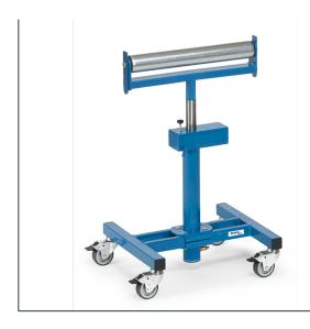
To support long materials on saws, presses, drills etc. Continuously adjustable in height, rotatable and lockable, with pneumatic lowering damping. Mobile. Supporting roller of tubular steel 60 mm Ø, 450 mm wide, ball bearing mounted. Loose gravity-stops on both sides 20 mm above top edge of roller (automatically turn away for wide work pieces). 4 swivel castors, all 4 with wheel locks. Flat packed for easy self assembly.
