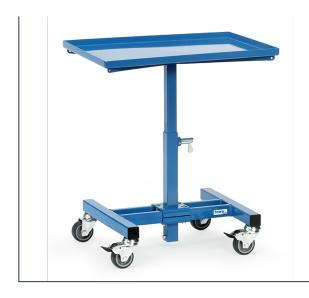
For plastic boxes, steel plate boxes, wire baskets etc., adjustable in height and mobile. Sectional steel-/ tubular construction with steel plate platform with all side rim 20 mm high. Not inclinable. Adjustable in height in intervals of 25 mm. Powder coating, blue RAL 5007. 4 swivel castors with TPE tyres, hubs with slide bearing. Brakes at 2 swivel castors according to the European Standard EN 1757-3 (safety of platform trolleys).
