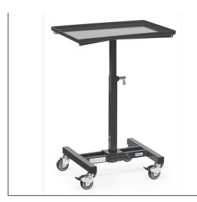
For plastic boxes, steel plate boxes, wire baskets etc., adjustable in height and mobile. Sectional steel-/ tubular construction with steel plate platform. Powder-coated anthracite grey RAL 7016. 4 swivel castors with TPE tyres, hubs with bush bearing, 2 swivel castors with wheel locks. Steel plate platform with all side rim, 20 mm high. Not inclinable, adjustable in height in intervals of 25 mm.
