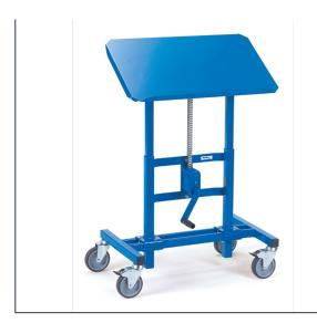
For plastic boxes, steel plate boxes, wire baskets etc., adjustable in height and mobile. Sectional steel-/ tubular construction with steel plate platform. Powder-coated blue RAL 5007. 4 swivel castors with TPE tyres, hubs with bush bearing, 2 swivel castors with wheel locks. Steel plate platform with single-sided lay-on edge, inclinable by 15° und 30°, continuously adjustable in height via rack and pinion jack , even under load. 2 telescopic pillars.
