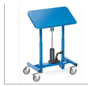
For plastic boxes, steel plate boxes, wire baskets etc., adjustable in height and mobile. Sectional steel-/ tubular construction with steel plate platform. Powder-coated blue RAL 5007. 4 swivel castors with TPE tyres, hubs with bush bearing, 2 swivel castors with wheel locks. Steel plate platform with single-sided lay-on edge, inclinable by 15° und 30°, continuously adjustable in height via hydraulic pump, even under load. Operated via pedal, precisely adjustable via lowering valve.
