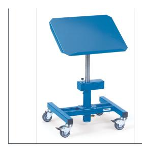
For plastic boxes, steel plate boxes, wire baskets etc., adjustable in height and mobile. Sectional steel-/ tubular construction with steel plate platform. Powder-coated blue RAL 5007. 4 swivel castors with TPE tyres, hubs with bush bearing, 2 swivel castors with wheel locks. Steel plate platform with single-sided lay-on edge, inclinable by 15° and 30°, continuously adjustable in height, rotatable and lockable, with pneumatic lowering damping.
