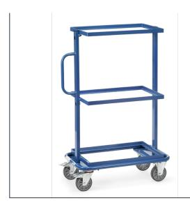
Tubular steel and steel section construction, powder coated. With open frames without board. Capacity upper and middle shelf 50 kg. 2 swivel and 2 fixed-wheel castors, TPE tyres, 125 x 32 mm, hubs with groove ball bearing. Swivel castors with wheel lock, according to European Standard EN1757-3 (safety of platform trolleys).
